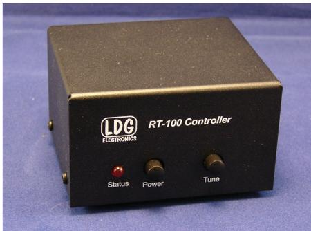
**Important Note:** The transmission line between the RC-100 and the RT-100 tuner must never be grounded. Doing so would cause the RC-100 to attempt to source 12 vdc directly to ground, damaging the unit. Never use coax switches that ground unselected ports even momentarily.
